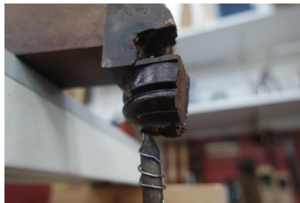
Figure 14 Application of heat into adhered join using soldering iron and wire.
